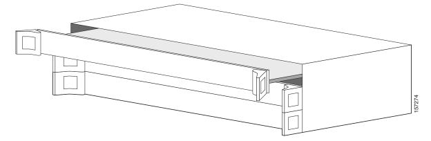
**Step 7** Use even pressure to push the module further into the slot.
